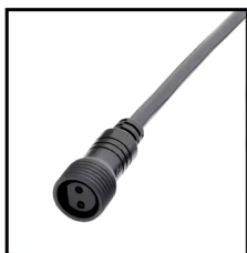
IP67 Connector 2PIN Order Code: 7601515-05 Wire gauge: 0.326mm 2 /22AWG Protection: IP67 (Mated) Connector type : Female
