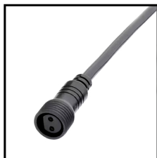
IP67 Connector 2PIN Order Code: 7601220-05 Wire gauge: 0.326mm 2 /22AWG Protection: IP67 (Mated) Connector type : Female
