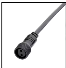
IP67 Connector 2PIN Order Code: 7601212-05 Wire gauge: 0.326mm 2 /22AWG Protection: IP67 (Mated) Connector type : Female
