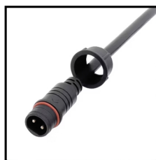
IP67 Connector 2PIN Order Code: 6301515-04 Wire gauge: 0.326mm 2 /22AWG Protection: IP67 (Mated) Connector type : Male
