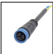
IP67 Connector 3PIN Order Code: 6331515-05 Wire gauge: 0.326mm 2 /22AWG Protection: IP67 (Mated)
