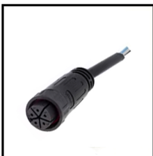
IP67 Connector 5PIN Order Code: 6361515-05 Wire gauge: 0.326mm 2 /22AWG Protection: IP67 (Mated)
