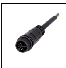
IP67 Connector 5PIN Order Code: 6321515-04 Wire gauge: 0.326mm 2 /22AWG Protection: IP67 (Mated)
