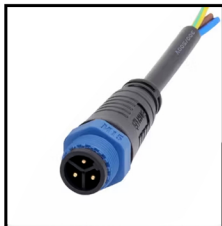
IP67 Connector 3PIN Order Code: 6171515-04 Wire gauge: 0.326mm 2 /22AWG Protection: IP67 (Mated)
