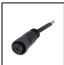
IP67 Connector 5PIN Order Code: 6351515-05 Wire gauge: 0.326mm 2 /22AWG Protection: IP67 (Mated)
