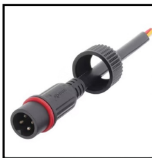
IP67 Connector 4PIN Order Code: 6311515-04 Wire gauge: 0.326mm 2 /22AWG Protection: IP67 (Mated) Connector type : Male
