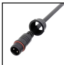
IP67 Connector 2PIN Order Code: 6381515-04 Wire gauge: 0.326mm 2 /22AWG Protection: IP67 (Mated)
