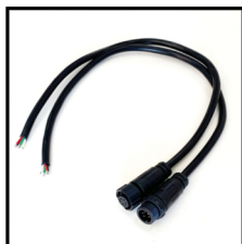
IP67 Connector 2PIN Digital Order Code: 8701520-05 Wire gauge: 0.326mm 2 /22AWG Protection: IP67 (Mated)
