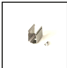
Mounting Clips Order Code: 8700816-03 Dimension: L30*W10*H17mm Material: stainless steel Color: silver Each meter led strips needs 2 clips + 2 screws
