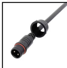
IP67 Connector 2PIN Order Code: 8700714-04 Wire gauge: 0.326mm 2 /22AWG Protection: IP67 (Mated) Connector type : Male
