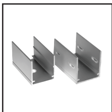
Mounting Clips Order Code : 8700614-03 Dimension : L20xW7.9xH15.6mm Material : Stainless steel Color : Silver Each meter led strips needs 2 clips + 2 screws
