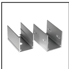
Mounting Clips Order Code : 8700612-03 Dimension : L20*W7.9*H13.6mm Material : stainless steel Color : silver Each meter led strips needs 2 clips + 2 screws
