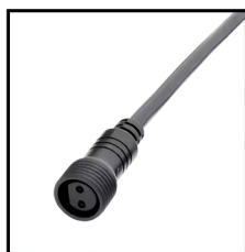
IP67 Connector 2PIN Order Code: 8700408-05 Wire gauge: 0.326mm 2 /22AWG Protection: IP67 (Mated) Connector type : Female
