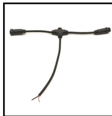
IP67 T Type Connector Order Code: 8731520-08 Wire Gauge: 0.326mm 2 /22AWG Protection: IP67 (Mated)
