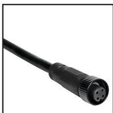
IP67 Connector 4PIN Order Code : 8711018-05 Wire gauge : 0.326mm 2 /22AWG Protection : IP67 (Mated) Connector type : Female
