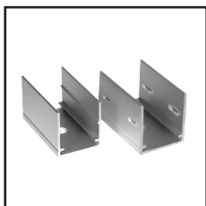
Mounting Clips Order Code : 8711018-03 Dimension : L30xW12.2xH16mm Material : Stainless steel Color : Silver Each meter led strips needs 2 clips + 2 screws
