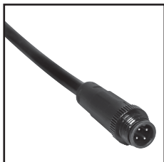
IP67 Connector 4PIN Order Code : 8711018-04 Wire gauge : 0.326mm 2 /22AWG Protection : IP67 (Mated) Connector type : Male
