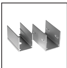
Mounting Clips Order Code : 8721018-03 Dimension : L30xW12.2xH16mm Material : Stainless steel Color : Silver Each meter led strips needs 2 clips + 2 screws
