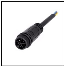
IP67 Connector 5PIN Order Code: 8761616-04 Wire gauge: 0.326mm 2 /22AWG Protection: IP67 (Mated)
