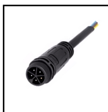
IP67 Connector 5PIN Order Code: 8761520-04 Wire gauge: 0.326mm 2 /22AWG Protection: IP67 (Mated)
