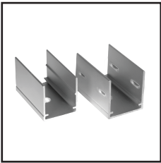
Mounting Clips Order Code : 8761220-03 Dimension : L30*W14*H22.5mm Material : stainless steel Color : silver Each meter led strips needs 2 clips + 2 screws
