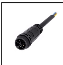
IP67 Connector 5PIN Order Code: 8760816-04 Wire gauge: 0.326mm 2 /22AWG Protection: IP67 (Mated)
