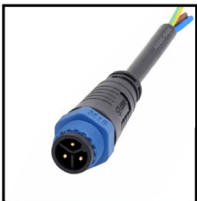
IP67 Connector 3PIN Order Code: 8771220-04 Wire gauge: 0.326mm 2 /22AWG Protection: IP67 (Mated)
