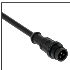
IP67 Connector 3PIN Order Code : 8771020-04 Wire gauge : 0.326mm 2 /22AWG Protection : IP67 (Mated) Connector type : Male
