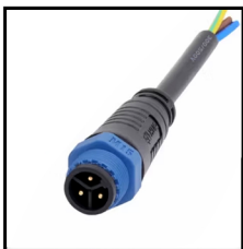
IP67 Connector 3PIN Order Code: 8770816-04 Wire gauge: 0.326mm 2 /22AWG Protection: IP67 (Mated)
