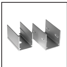
Mounting Clips Order Code : 8770614-03 Dimension : L20xW7.9xH15.6mm Material : Stainless steel Color : Silver Each meter led strips needs 2 clips + 2 screws
