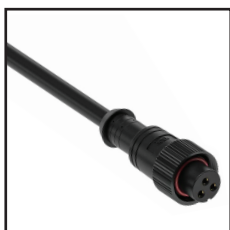
IP67 Connector 3PIN Order Code : 8770614-05 Wire gauge : 0.326mm 2 /22AWG Protection : IP67 (Mated) Connector type : Female
