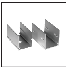
Mounting Clips Order Code : 8751520-03 Dimension : L30*W15*H20mm Material : stainless steel Color : silver Each meter led strips needs 2 clips + 2 screws
