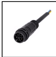
IP67 Connector 5PIN Order Code: 8750816-04 Wire gauge: 0.326mm 2 /22AWG Protection: IP67 (Mated)
