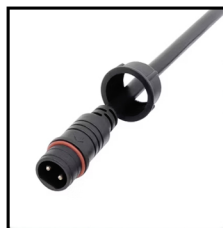
IP67 Connector 2PIN Order Code: 8781515-04 Wire gauge: 0.326mm 2 /22AWG Protection: IP67 (Mated)
