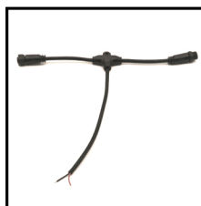
IP67 T Type Connector Order Code: 8781020-08 Wire Gauge: 0.326mm 2 /22AWG Protection: IP67 (Mated)
