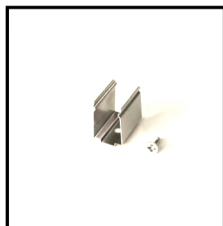
Mounting Clips Order Code: 8780816-03 Dimension: L30*W10*H17mm Material: stainless steel Color: silver Each meter led strips needs 2 clips + 2 screws
