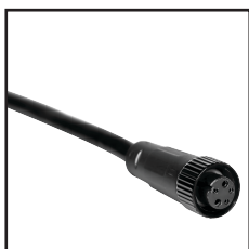
IP67 Connector 5PIN Order Code : 8791520-05 Wire gauge : 0.326mm 2 /22AWG Protection : IP67 (Mated) Connector type : Female
