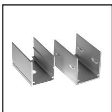
Mounting Clips Order Code : 8791520-03 Dimension : L30*W15*H20mm Material : stainless steel Color : silver Each meter led strips needs 2 clips + 2 screws
