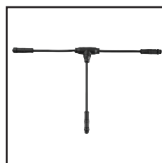
IP67 T Type Connector Order Code : 8791520-08 Wire Gauge : 0.326mm 2 /22AWG Protection : IP67 (Mated)
