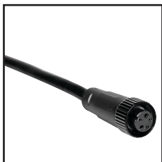
IP67 Connector 5PIN Order Code : 8791515-05 Wire gauge : 0.326mm 2 /22AWG Protection : IP67 (Mated) Connector type : Female
