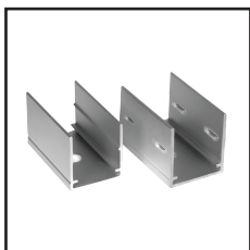
Mounting Clips Order Code : 8791515-03 Dimension : L20*W16.6*H12.4mm Material : stainless steel Color : silver Each meter led strips needs 2 clips + 2 screws
