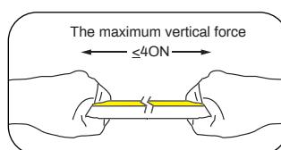
The safe tensile force for the LED strip shall be  $\leq 4\text{ON}$
