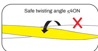
The safe twisting angle for the LED strip shall not exceed 180°.
