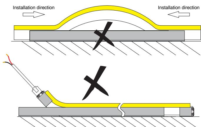
Ensure the feeding cable not bear force, keep the head 10mm in natural loose. ← →
