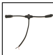
IP67 T Type Connector Order Code: 8791020-08 Wire Gauge: 0.326mm 2 /22AWG Protection: IP67 (Mated)
