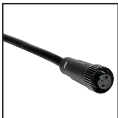
IP67 Connector 5PIN Order Code : 8791018-05 Wire gauge : 0.326mm 2 /22AWG Protection : IP67 (Mated) Connector type : Female
