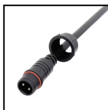
IP67 Connector 2PIN Order Code: 7301020-04 Wire gauge: 0.326mm 2 /22AWG Protection: IP67 (Mated) Connector type : Male
