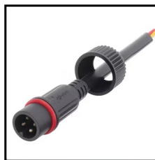
IP67 Connector 4PIN Order Code: 7311020-04 Wire gauge: 0.326mm 2 /22AWG Protection: IP67 (Mated) Connector type : Male
