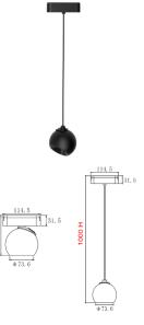
GLOB'B Is Decorative Magnetic track light installed on Low Voltage Magnetic Track.
