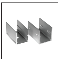
Mounting Clips Order Code : 8721515-03 Dimension : L20*W16.6*H12.4mm Material : stainless steel Color : silver Each meter led strips needs 2 clips + 2 screws
