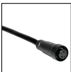
IP67 Connector 5PIN Order Code : 8721515-05 Wire gauge : 0.326mm 2 /22AWG Protection : IP67 (Mated) Connector type : Female
