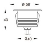
CRYPT is wood floor thin inground light typically feature durable, weather-resistant housings suitable for outdoor use. Excellent heat dissipation.
