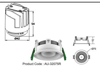
Die Cast Aluminum Body and Frame with SS Clips
