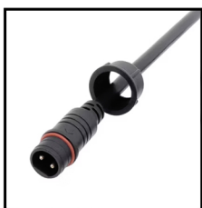
IP67 Connector 2PIN Order Code: 8903525-04 Wire gauge: 0.326mm 2 /22AWG Protection: IP67 (Mated) Connector type : Male
