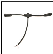
IP67 T Type Connector Order Code: 8901207-08 Wire Gauge: 0.326mm 2 /22AWG Protection: IP67 (Mated)
