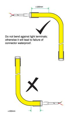
Ensure the feeding cable not bear force, keep the head 10 mm in natural loose.
