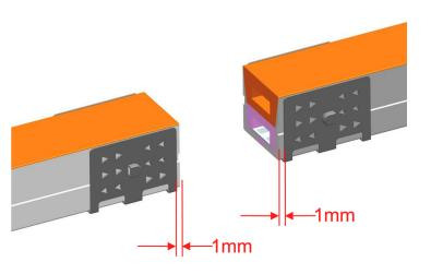
Note: The install distance between buckle and cutting section is ± 1mm
