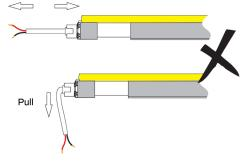
Mount the cable junction in hermetic enclosure like waterproof junction box in outdoor application.
