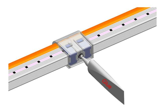
If the strips need to be IP67 waterproof rated, please make sure the connector installed correctly, strip lights up properly. Then pour the glue to the injection port, until the gule fills the entire connector and overflows to the surface of strip. Once glue injected OK, wait for 3-5 hours to make it IP67 waterproof rated.
