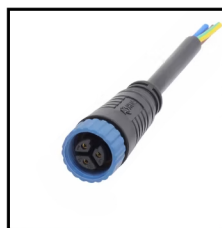
IP67 Connector 3PIN Order Code: 8931010-05 Wire gauge: 0.326mm 2 /22AWG Protection: IP67 (Mated)
