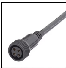
IP67 Connector 4PIN Order Code: 8911818-05 Wire gauge: 0.326mm 2 /22AWG Protection: IP67 (Mated) Connector type : Female
