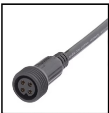
IP67 Connector 4PIN Order Code: 8911616-05 Wire gauge: 0.326mm 2 /22AWG Protection: IP67 (Mated) Connector type : Female
